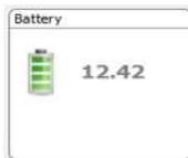
**Battery level indicator:** In case of low battery, the color of the icon changes. A fully charged battery is between 12.8V and 13.1V
