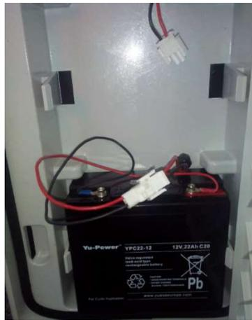
**Power autonomy** – Two batteries will last an average of 7 days depending on luminosity and traffic flow. Do not mount or un-mount the radar until you have removed the batteries first for both security and weight reasons. The radar will indicate low-battery by showing a tri-colored square on the bottom right corner of the speed display. At this time, the batteries should be replaced with the two charged batteries.
