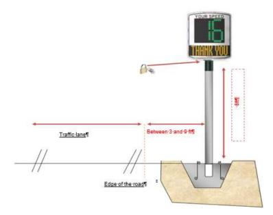
Do not install your sign at intersections or on bridges. It should be at least 500 ft away from cross traffic, since vehicles arriving from the side may be recorded as oncoming vehicles occasioning an issue with the traffic data.
