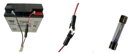
An 8x32 8A time-delayed fuse is positioned at the battery output to protect the unit if the power supply polarity is reversed. A second fuse located inside the box also protects the unit.
